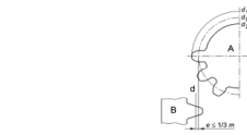
Key A pinion B rack d 1 outside diameter of pinion d 2 pitch diameter of pinion d 3 base diameter of pinion g pitch line of rack f 1/3 module max.
